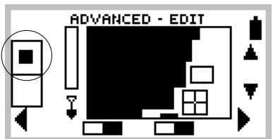
Figure 6.10 Edit screen with target crosshair and target frame
