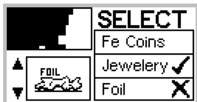
Figure 6.8 Edit screen with target frame
