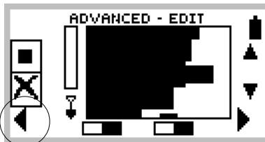
Figure 6.12 Target frame dragged to complete discrimination pattern
